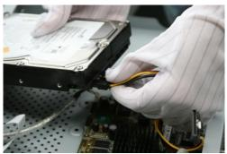
**3.** Connect the power cable to the HDD.
