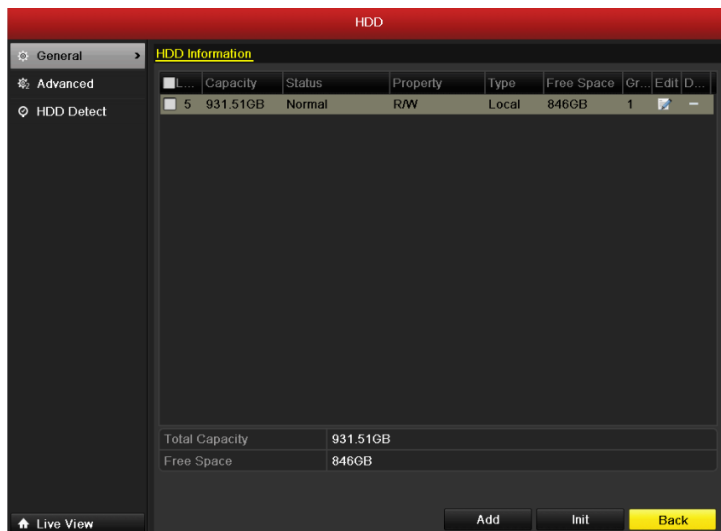
Figure 10.4HDD Status Changes to Normal
