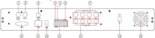
Fig 2.5 Rear Panel for 4-ch
