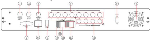
Fig 2.6 Rear Panel for 8-ch
