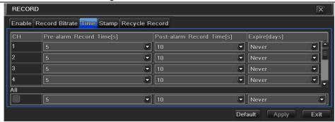
Fig 4-13 record configuration-time
