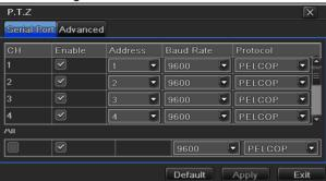
Fig 4-36 P.T.Z configuration-serial port
