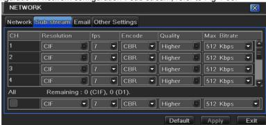
Fig 4-30 network configuration-sub stream
