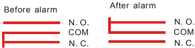
Fig 2.9 Relay Output Status
